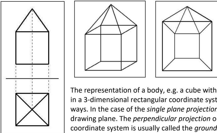
The representation of a body, e.g. a cube with an attached half octahedron, in a 3-dimensional rectangular coordinate system can be done in different ways. In the case of the *single plane projection*, an object is projected onto a drawing plane. The *perpendicular projection* onto the  $x$ - $y$ -plane in a coordinate system is usually called the *ground plan*, the projection onto the  $y$ - $z$ -plane is called the *elevation*, and the projection onto the  $x$ - $z$ -plane is
