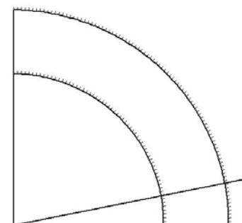
Such a system is pictured on the left-hand side of the Portuguese postage stamp from 1978, labelled "O NONIO." The diagram above serves as an illustration of the method of measurement: The marker passes quite precisely through the eighth demarcation point of the quarter-circle with 63 equal segments. Therefore, the included angle is equal to  $8/63 \cdot 90^\circ (\approx 11.43^\circ)$ .
